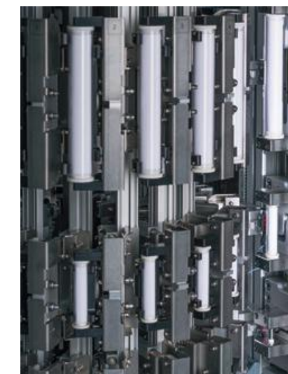
Column carousel is in the rear position with locked columns in the column tower.
