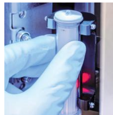
Insertion of columns - sensors check, if columns match with method input
