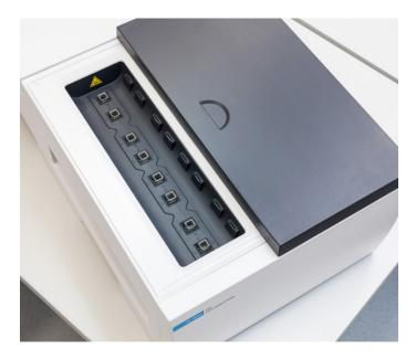
Figure 1. The sample compartment of the Cary 3500 Multizone UV-Vis spectrophotometer has a built-in multicell holder. Each sample/reference pair can be held at a different temperature.
