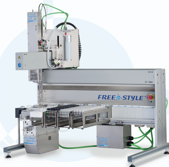
Robotic system FREESTYLE for new automated QuEChERS method
