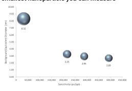
The relationship between calculated background equivalent diameter and instrument sensitivity (cps/ppb) for the analyte element.
